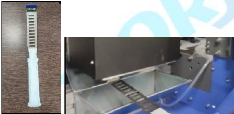
Figure 49: Cleaning the Print Head with a head wiper( reference image)
