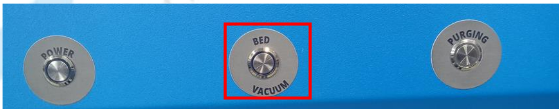
Figure 16: Turning ON the Bed Vacuum Button
