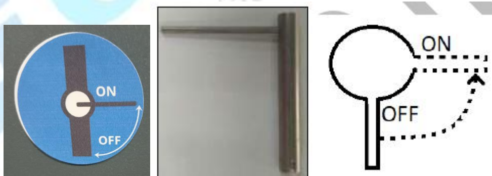
Figure 13: Opening Ink Valve Using the Key
