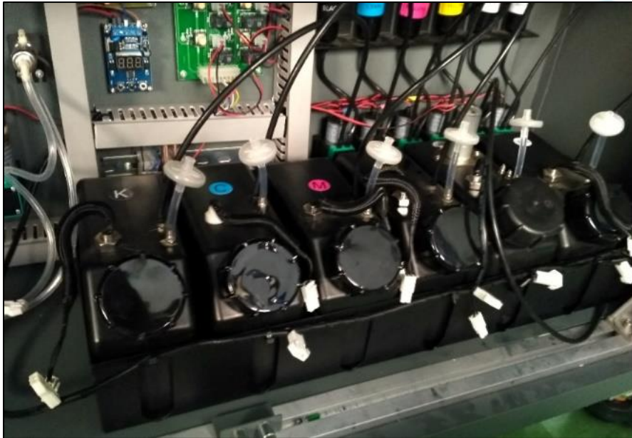
Figure 17 Main Ink Tanks and their Connectors
