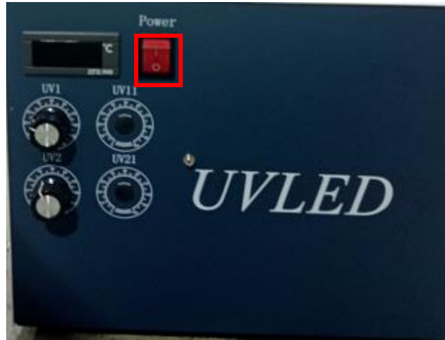
Figure 10: Switch ON UV Lamps
