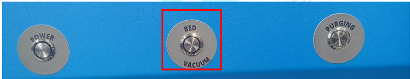
Figure 11: Turning On the Bed Vacuum Button
